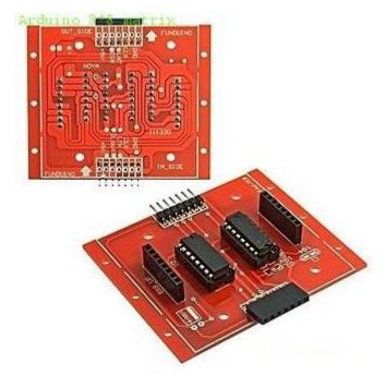
The 8\*8 lattice drive module developed by KEYE team is equipped with high-speed 74HC595 deserializer chip. Only 3 signal lines are needed to drive 8\*8 dot matrix screen, saving your valuable I/O resources in Arduino controller to maximum extent.
